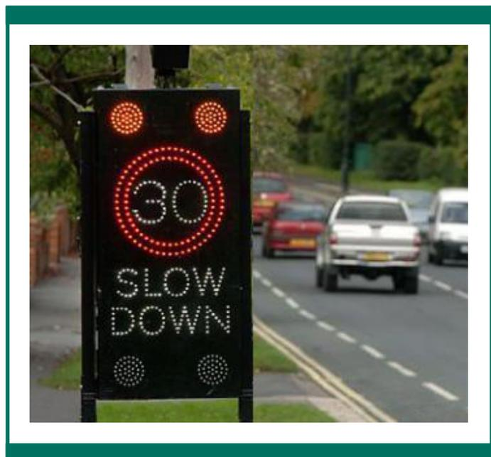
Figure 3 Vehicle activated VMS with flashing amber lamps
