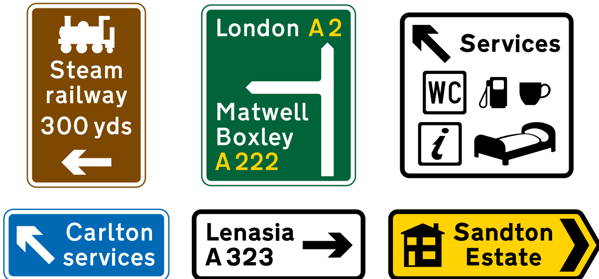
Figure 4-4 Informatory, Directional and Tourist Signs
