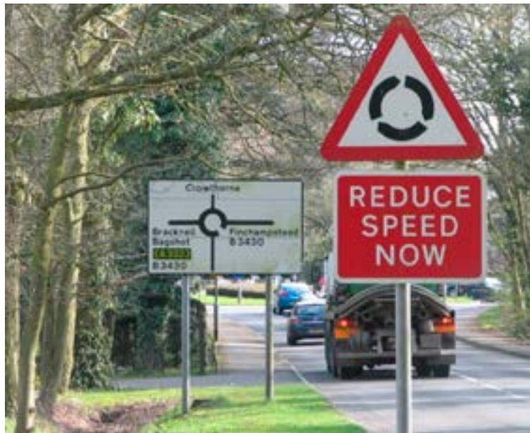
Figure 2-1 Overuse of warning signs – this roundabout on a single carriageway road is adequately indicated by the map-type advance direction sign
